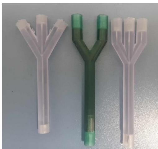
Fig. 53 The final 3D printed microfluidic devices
