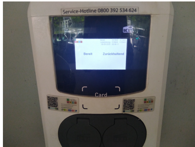
Figure 2.8: The message showing on the monitor of the charging station that it has been reserved. From [Bas+19].
