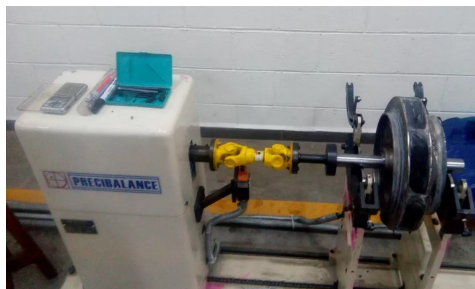
Figure 2.3: End drive balancing machine with universal shaft coupling [13]
