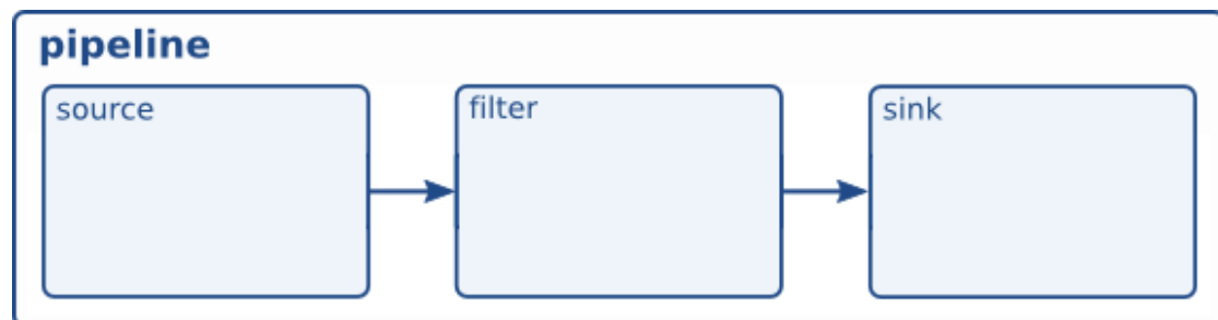
■ Figure 2.2 Simple GStreamer pipeline obtained from the official Gstreamer website [19]
