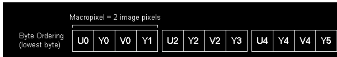
■ Figure 3.1 UYVY color format illustration acquired from website [23]
