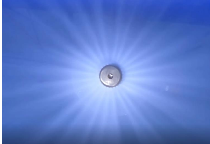
Figure 6.5 Oxidizer only cold flow
