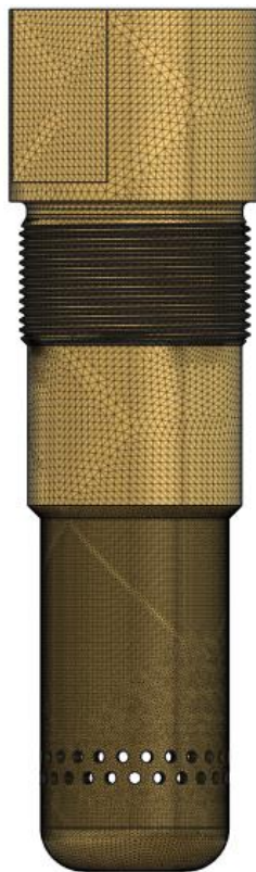
Figure 5.1 Pintle FEM analysis mesh
