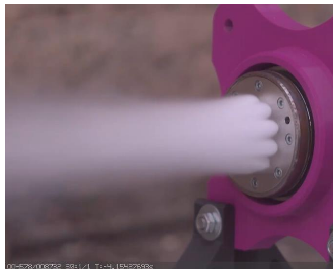
Figure 6.1 Hybrid injector cold flow test [2]
