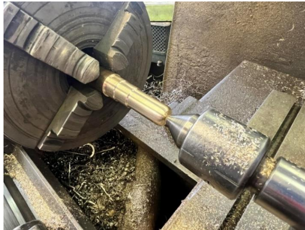
Figure 3.5 Manufacturing of the first pintle prototype from brass
