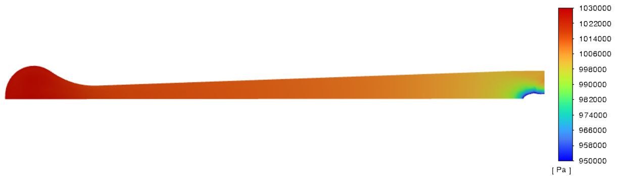
Figure 5.23 Manifold pressure losses
