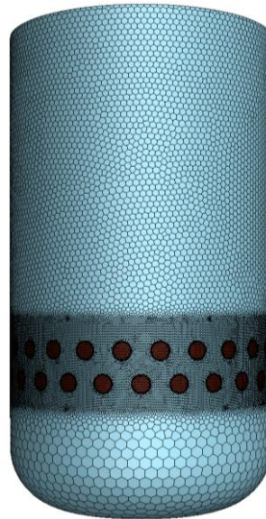
Figure 5.12 Pintle CFD mesh
