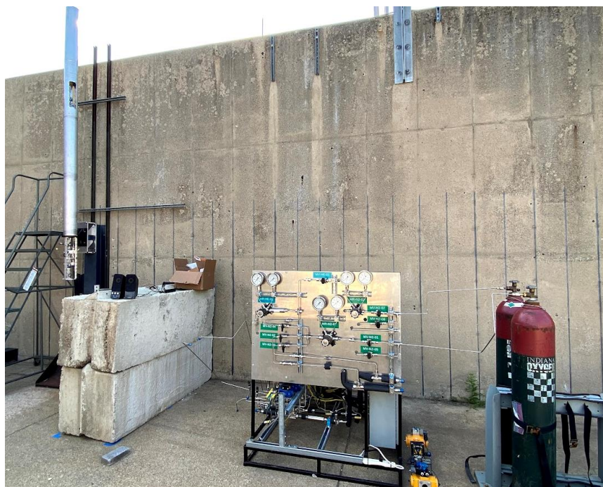
Figure 1.2 Purdue Space Programme Liquids GSE [15]
