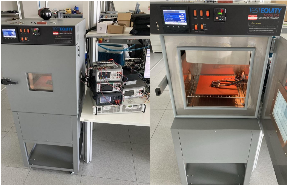
Figure 60: Measuring setup (left), detail of the temperature chamber (right)
