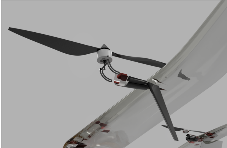
■ Figure 5.3 Convertiplane mechanism proposal
