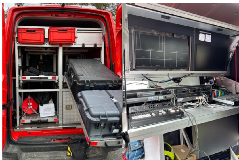
■ Figure 1.9 Transport van with specialised cargo shelves and video feed mixing station (authors archive)
