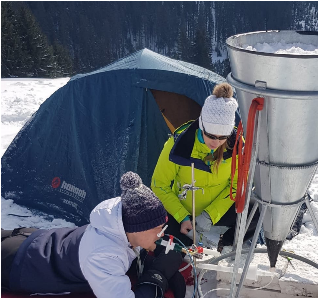
Figure 5.2 A photo from the stabilisation phase of the experiment. Subject is in a prone position, lying on an insulated mat, breathing through a mouthpiece connected to a monitor. The specially designed tubing is ready to be connected to the cone-shaped container filled with material simulating avalanche snow. The subject is monitored closely by the physician.
