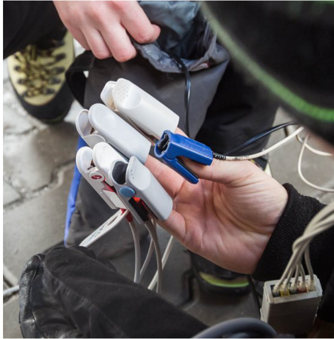
Figure 4.3 Subject's right hand with finger probes of five different pulse oximeters. The hand was placed in preheated insulated glove (in the assistant's hand on the photo).
