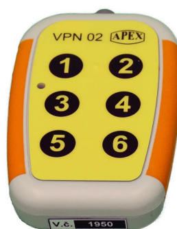
Figure 3.1: VPN transmitter used by visually impaired to activate audio signals. Source: [25]
