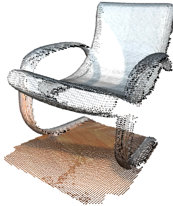
■ Figure 1.2 Point cloud representation of a chair scan [15].
