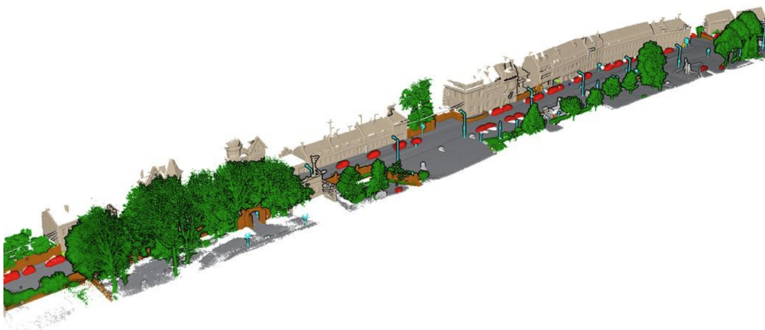
■ Figure 2.3 Example from the Lille NPM3D dataset [56]. Colors are semantic labels, where roads are gray, vehicles are red, buildings are beige, and vegetation is green.
