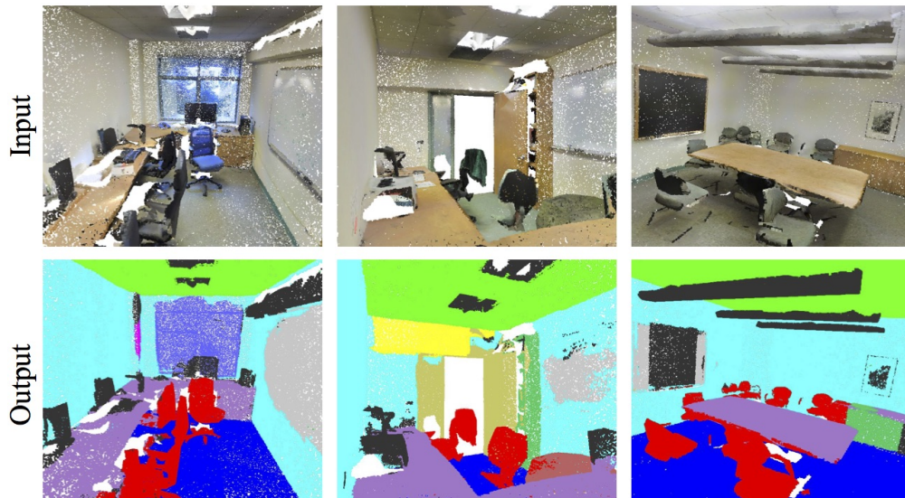
■ Figure 1.11 Example of semantic segmentation result from a neural network. The input consists of raw indoor point cloud data. The output is a segmented point cloud where different regions within the indoor space are highlighted [12].
