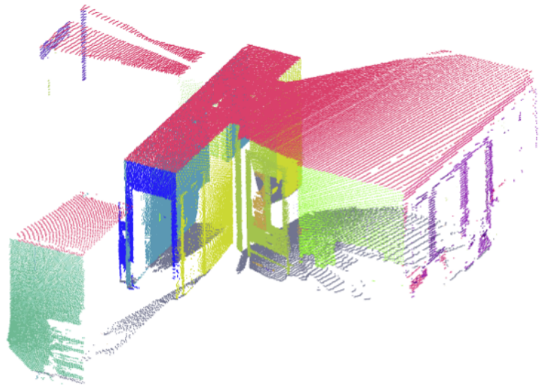
■ Figure 1.10 RANSAC used for plane detection on an indoor dataset. A different color marks different planes [24].
