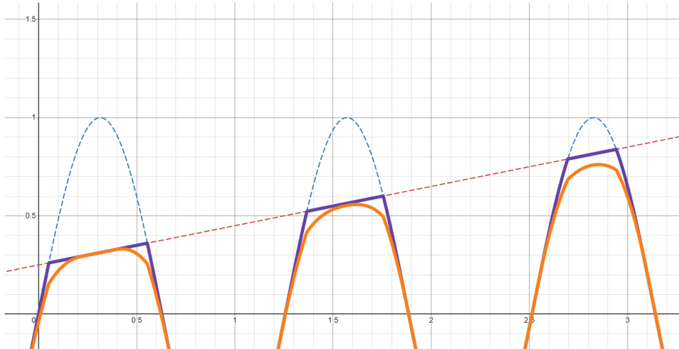
■ Figure 3.8 Example of smooth minimum function. Red and blue are initial functions, purple is the minimum of them, orange is the smooth minimum. Created in Desmos [33].
