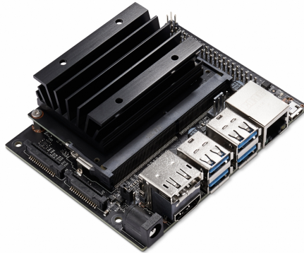
Figure 2.1: Jetson Nano Board Developer Kit [1].
