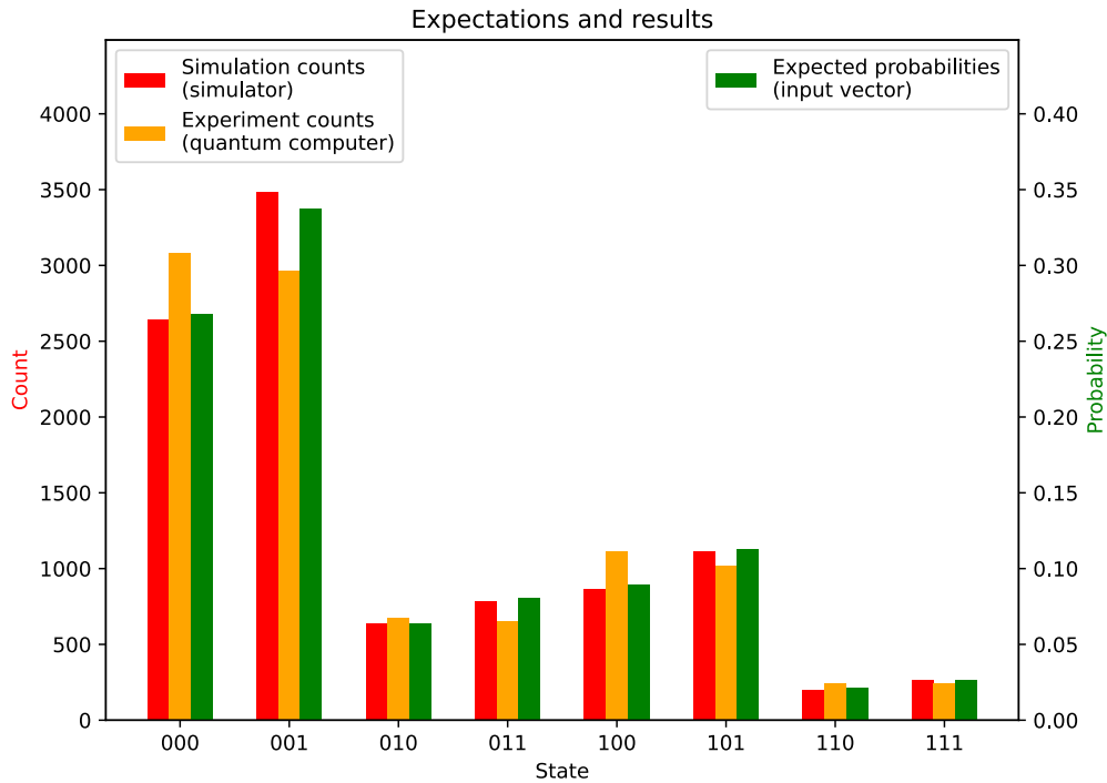
■ Figure 5.11 A histogram comparing the measurement outcomes of a simulation with the measurement results obtained by running a quantum circuit on the quantum computer ibm_osaka and the expected distribution of probabilities calculated from an input array. The values were obtained from a circuit created by using the implemented angle encoding method to encode the following input array: [0.74651424, 0.43896263, 0.5000283] .
