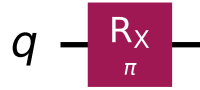
■ Figure 2.4 A visualization of the gate RX(\pi) applied to a qubit in a one-qubit quantum circuit created using the Qiskit library.
