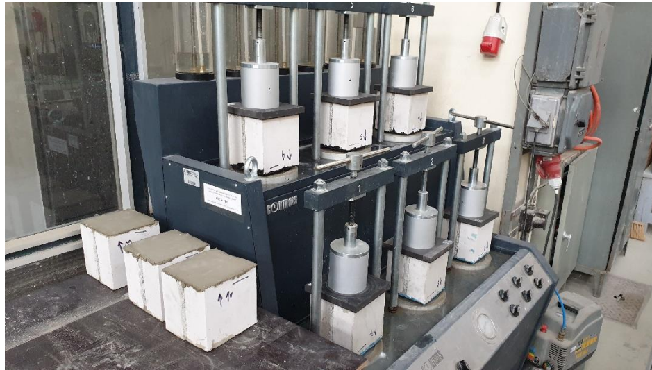
Figure 41: Water pressure test on the sets of specimens. Source: Author
