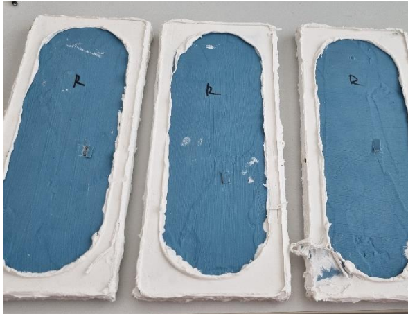
Figure 70. Specimens removed from the measuring device, sealant visible around the perimeter Source: Author
