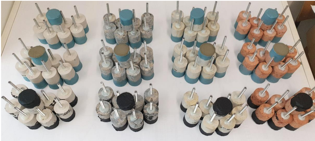
Figure 47: Finished set of specimens with the applied waterproofing screed (ceramics, concrete, lime sand, marl).
