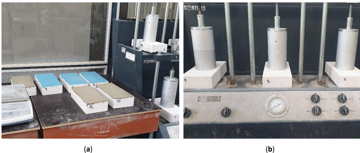
Figure 39. (a) Weighing the test specimens; (b) Water pressure test Source: Author
