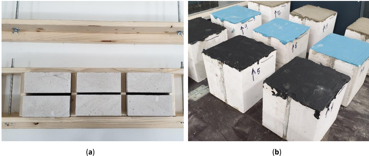
Figure 40: (a) Test specimen – lime-sand bricks and lime-cement mortar in wooden formwork; (b) Test specimens with applied waterproof screeds.
