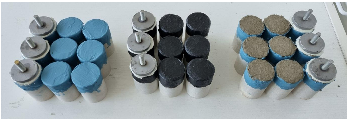
Figure 48: Finished set of specimens with the applied waterproofing screed (sandstone).
