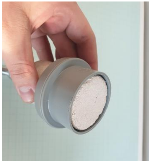
Figure 46: Prepared front of the test specimen for the application of a waterproofing screed Source: Author
