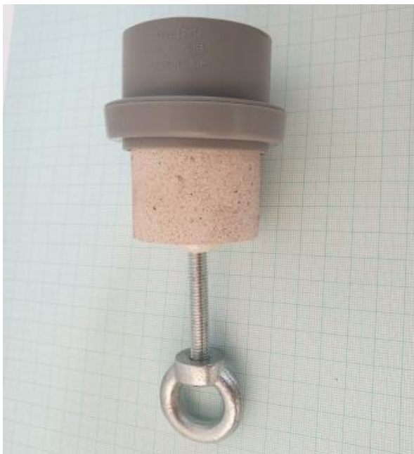
Figure 45: Prepared test specimen with glued threaded rod, PVC ring Source: Author
