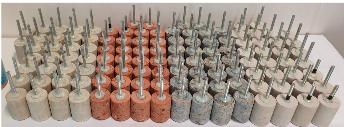
Figure 43: Assembly of all test specimens with glued threaded rods (ceramics, concrete, Lime sand, marl). Source: Author
