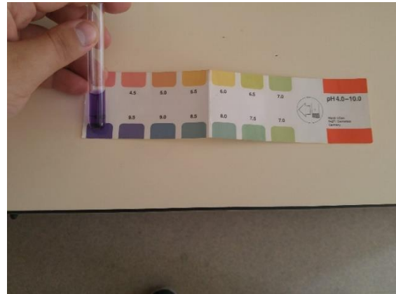
Figure 29: Colorimetric evaluation of pH by color and scale Source: Author
