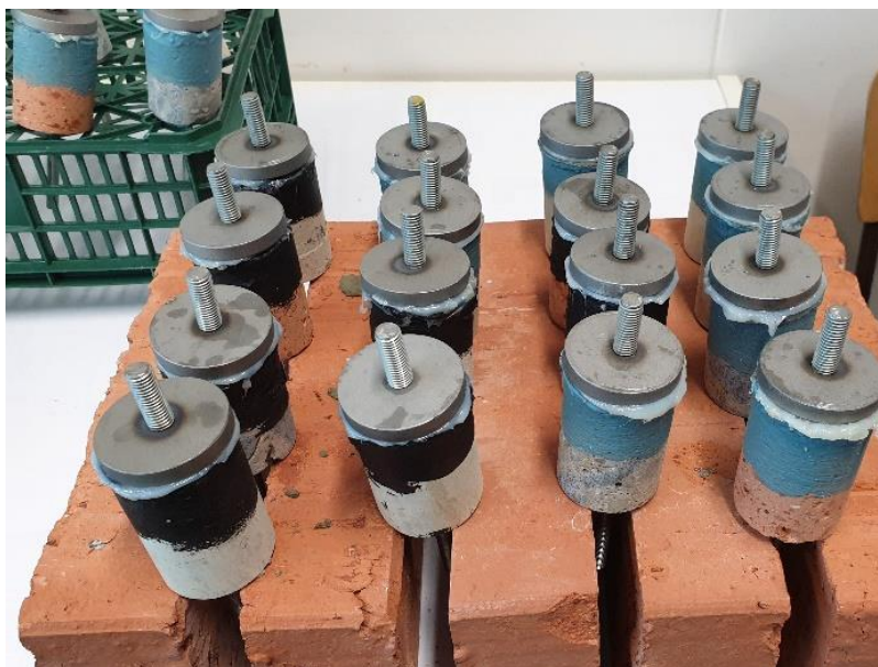
Figure 50: Gluing tear-off targets
