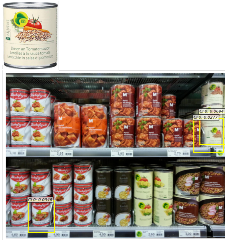
Figure 4.3: Detections for a class unseen in training. While the model has a general understanding of where the cans of lentils are located, the results are not quite accurate. The confidence scores are low too.
