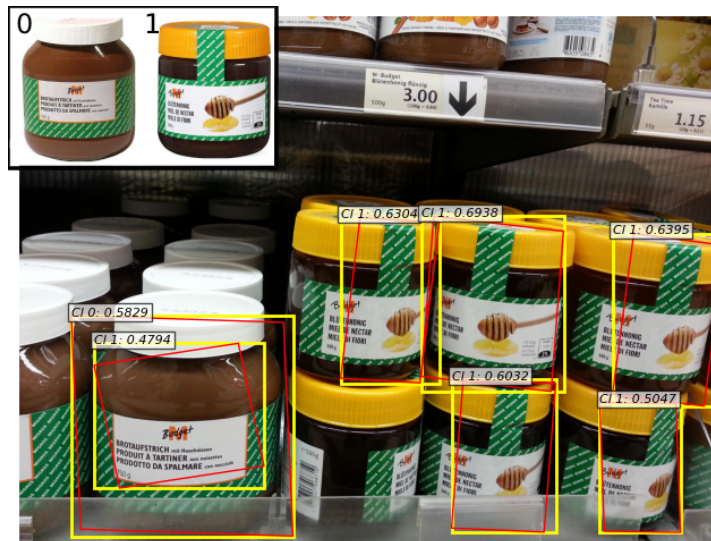
Figure 3.6: This example demonstrates a difficult case when objects are rotated in 3D space. Since the method matches the whole jar to the labels, the more the jars are rotated around their own axis, the more difficult it is to match them correctly.
