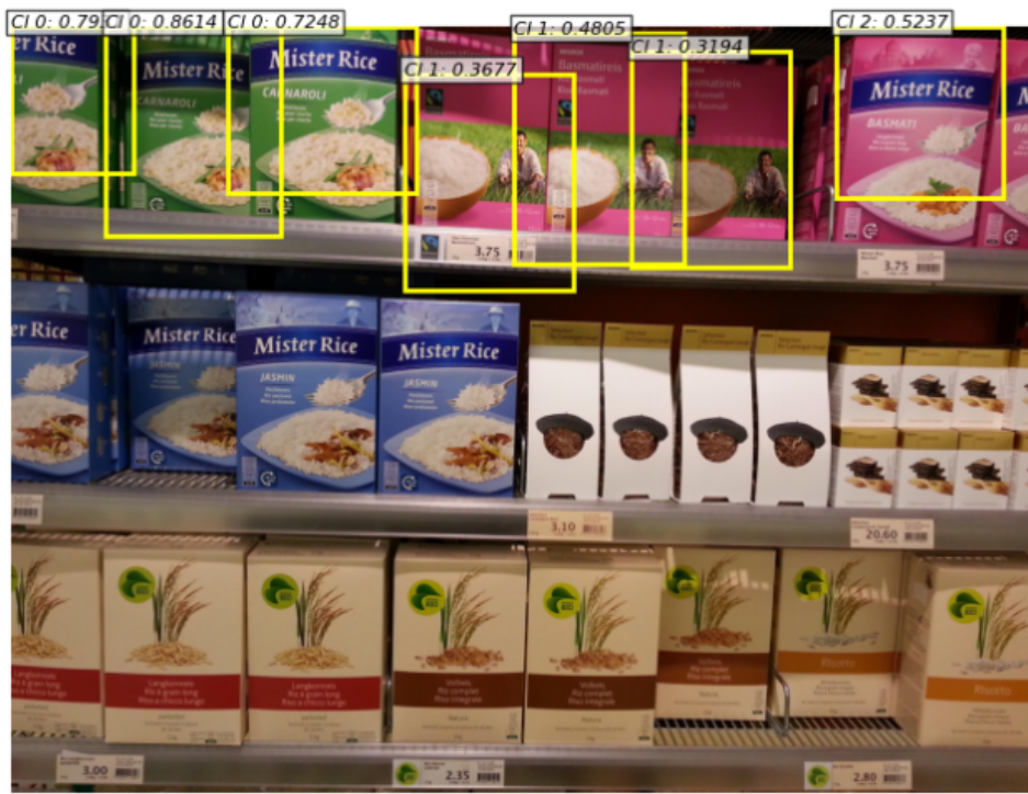
Figure 4.2: An example with rice boxes that were seen during the training. The class labels are correct, but the boxes are a little off and confidence scores are low for the 3 pink boxes in the middle.
