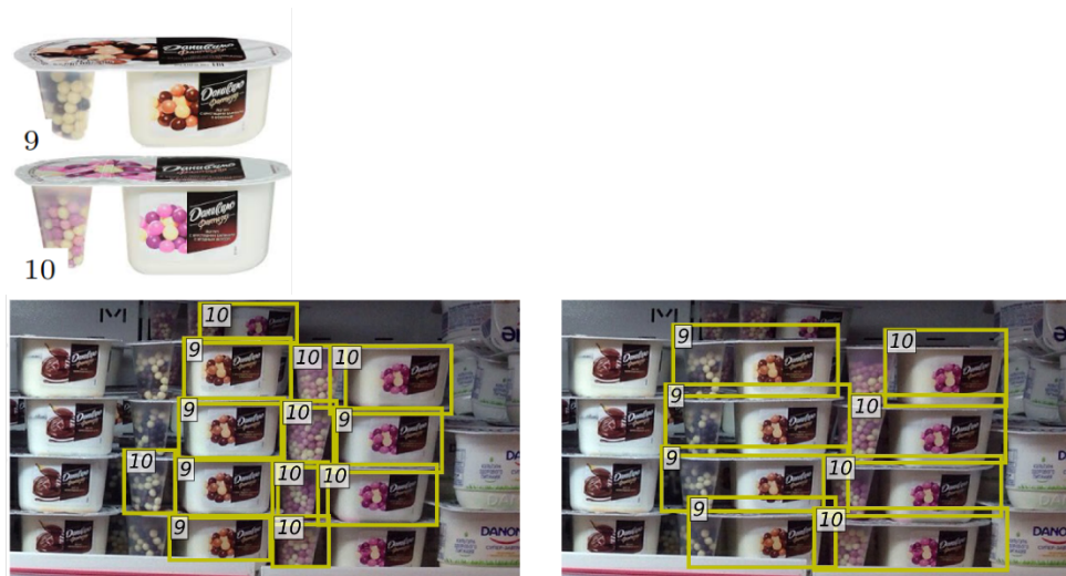
Figure 3.8: A qualitative comparison of OS2D model with a baseline similar to two-stage detectors (region detector + retrieval), for objects comprised of two parts and not seen during training. The baseline system has to finalize the object bounding box without knowing the classes of objects it is supposed to detect. Thus, if the object detector fails to detect two parts as one, the retrieval system cannot fix the boxes and recognize them correctly. On the other hand, the OS2D model is aware of the fact that the objects consist of two parts and detects them correctly. This image is borrowed from the paper[3]
