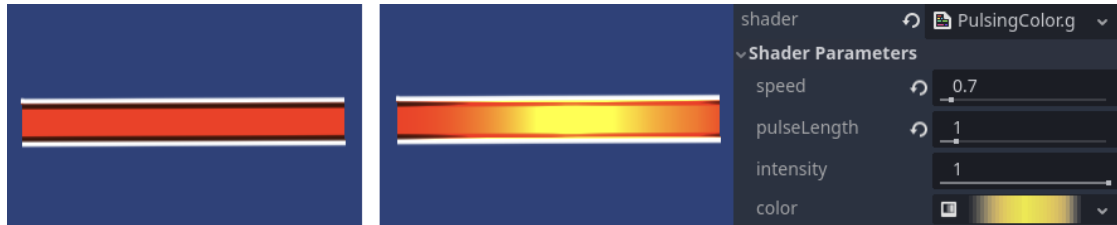
■ Figure 5.9 PulsingColor Shader, on the left the original visual, on the right with the shader applied
