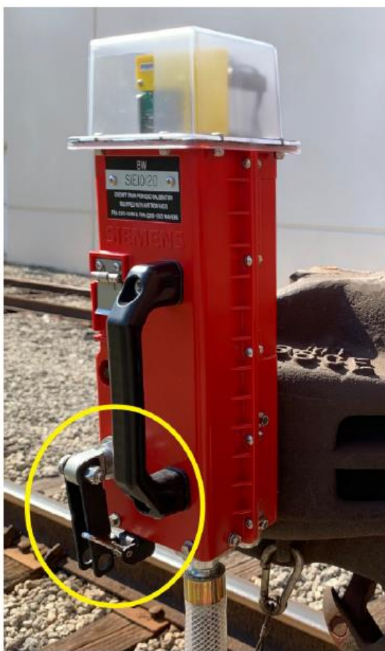
Figure 2-1 Unlatching the Crank Handle
