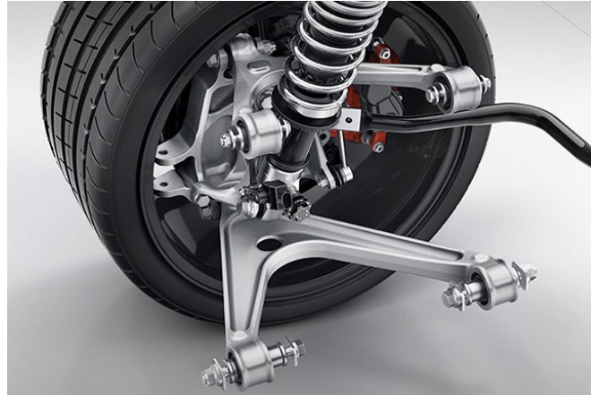
Figure 25 Double wishbone suspension example [14]
