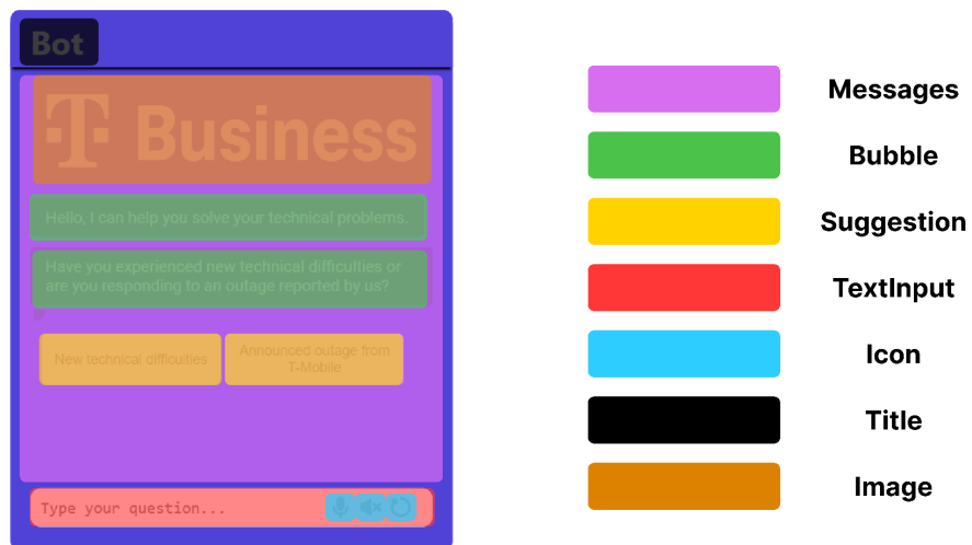
Figure 3.1: Different components marked on the UI
