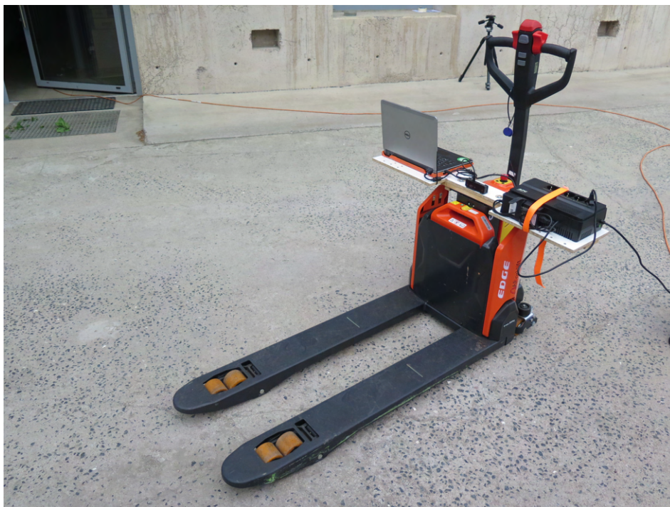
Figure 3.5: Pallet truck with all of our modifications.
