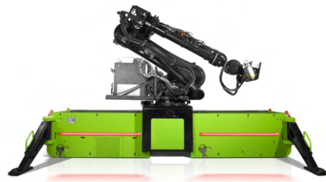
Figure 1.2: Automatic brick-laying robot [43]
