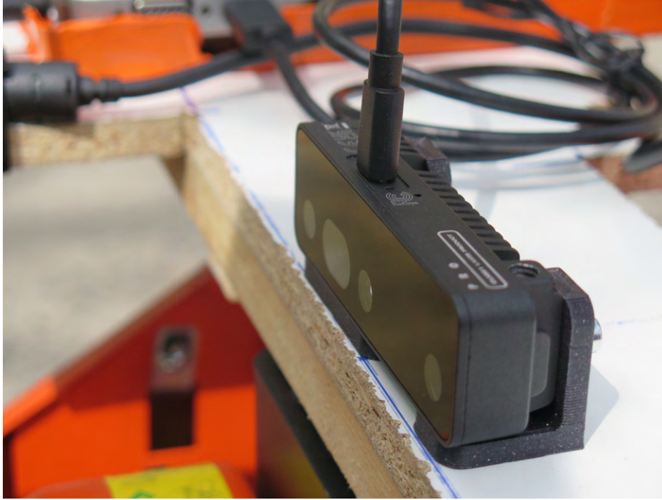
Figure 3.9: stereo camera in its mount
