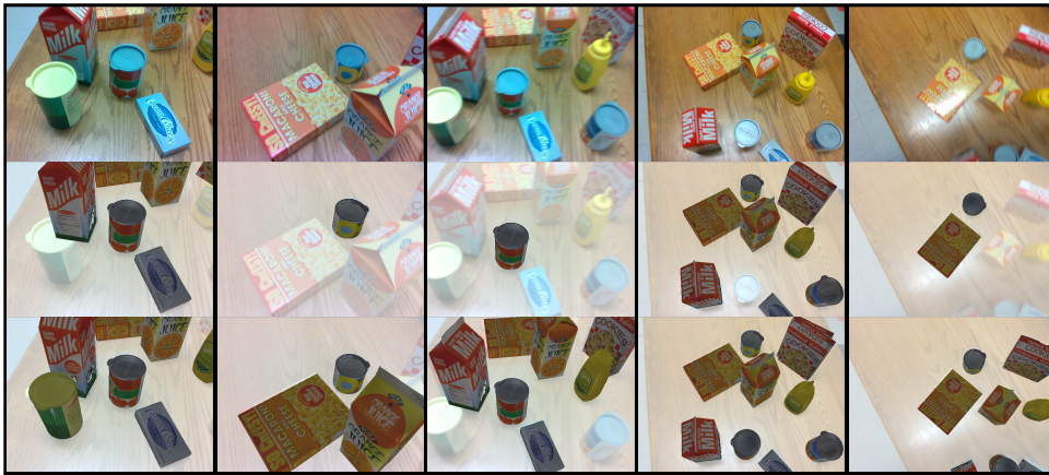
Figure 5.1: Example frames from HOPE-Video sequence are shown in the first row. The second row shows an overlay of the rendered poses predicted by the per-frame CosyPose [LCAS20] evaluation. It can be seen that some of the objects are not detected. Our temporally smoothed predictions are shown in the last row, mitigating the effect of missing detections.
