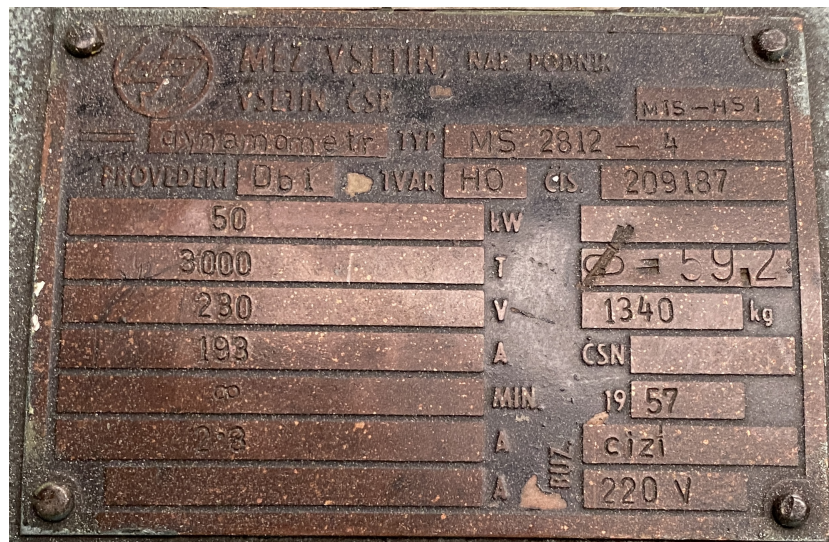
Figure 8.5: The rating plate of the used DM.
