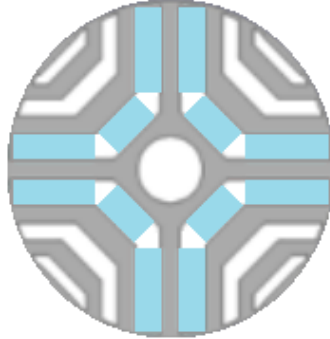
Figure 1.16: PM inserted into both d and q axes [38] (edited),
