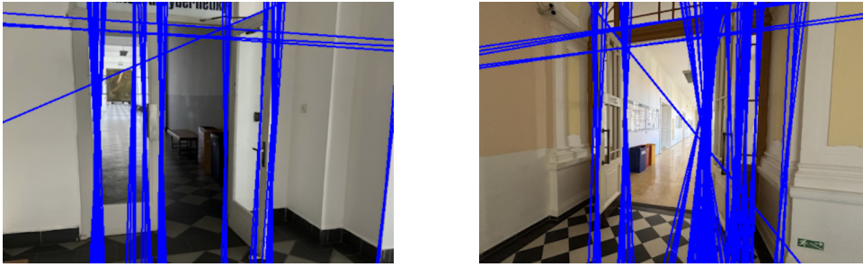
Figure 4.4: Output of the Hough Line Transform.
