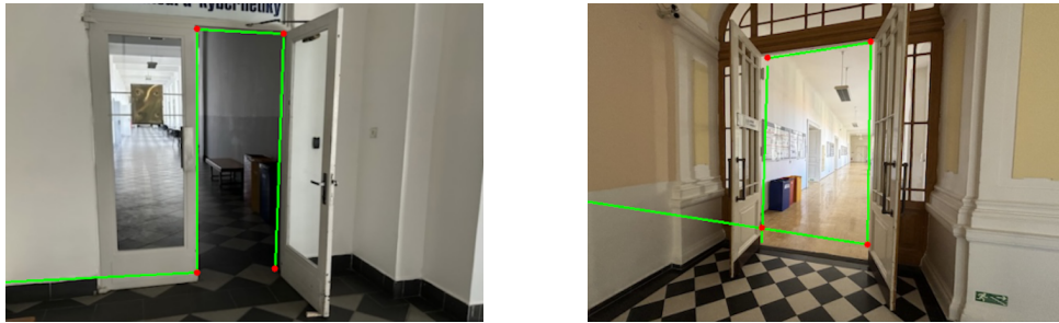
Figure 4.16: Determining corners through intersection line calculations.
