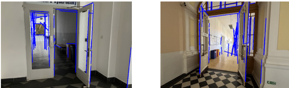
Figure 4.5: Output of the Probabilistic Hough Line Transform.
