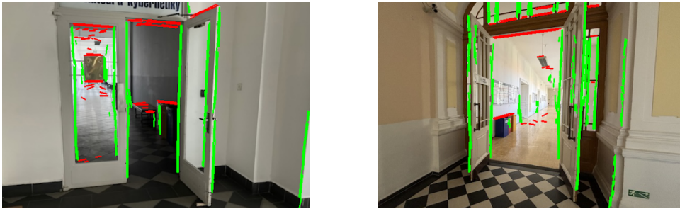
Figure 4.8: Result of filtering based on line angles.
