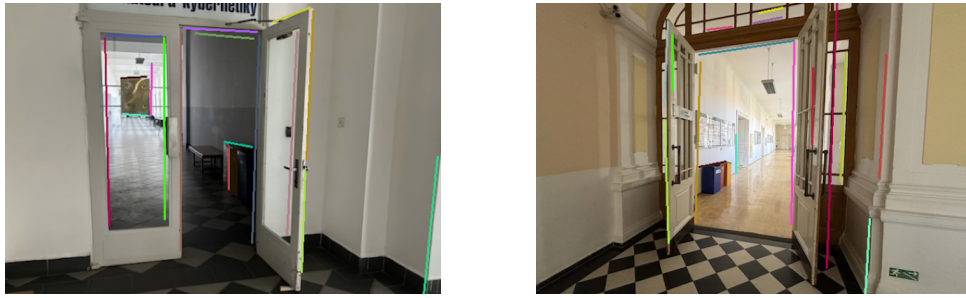
Figure 4.11: Lines fitted by the RANSAC algorithm.
