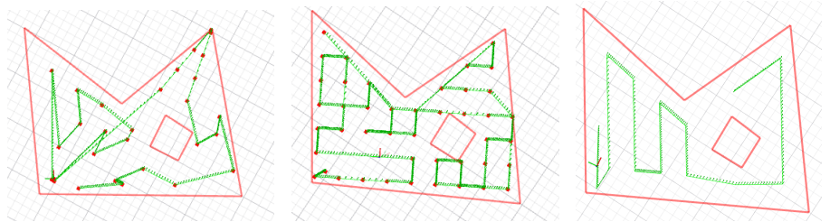
(a) Diagonal decomposition (b) Stride method (flow). (c) Morse decomposition (not flow).
