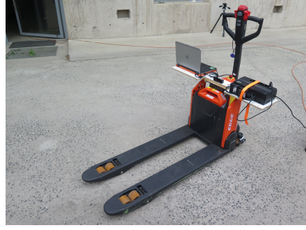
(b) : Pallet truck NOBLELIFT PTE20N mounted with RGBD camera, notebook and battery.
