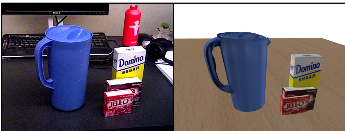
Figure 1.1: The left part of the image shows the input image taken from YCB-V dataset [1]. The right part of the image shows the object in estimated poses computed by MegaPose [2]. It is clearly visible that the objects in the estimated poses are colliding with each other and with the table.
