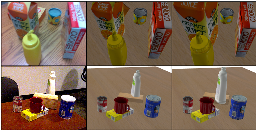
Figure 4.7: This figure shows examples of failure cases for our method. Input image is shown on the left, MegaPose predictions in the middle, and our refinement on the right. The first row shows the pizza box ( i.e. box behind the juice) in collision with the table and incorrectly rotated after the MegaPose prediction. During the optimization this incorrect prediction caused that the juice box is pushed towards the camera in order to resolve the collision. This can be seen in the last column of the first row, where refined juice box is bigger after rendering. In the second row, the wooden cube and the white bottle were predicted in a big collision by MegaPose. During our refinement, these two objects switch order compared to the input image.
