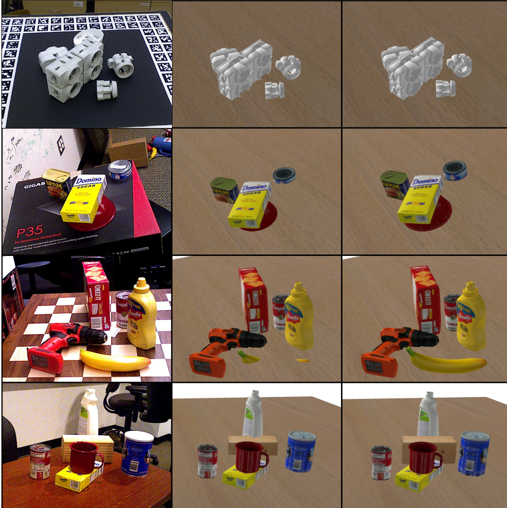
Figure 4.6: This figure shows a qualitative comparison of the initial poses estimated by MegaPose (middle column) and their subsequent refinement by our method (right column). The left column shows the images for which the estimation was performed. In the first row, notice the collision of the largest object in the middle with the floor, which was successfully resolved by our method. In the second row, all objects except the sugar box are in collision with the floor for MegaPose estimates. In the third row, the can and banana are in collision with the table. Also, notice the incorrectly estimated orientation of the banana. Although our method resolves the collision, the orientation of the banana is not changed and remains incorrect after our refinement, since a change of the orientation is not needed for the collision to be resolved. In the last row, there is a large collision between the wooden cube and the floor, and also between the cube and the white bottle; all resolved by our method.
