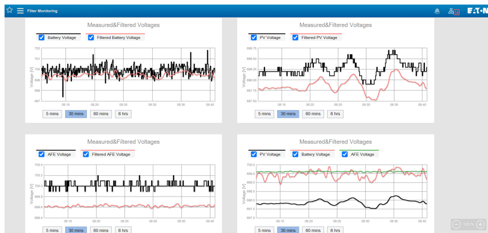
Figure 3.12: The graph of the measured and filtered voltages on the DC-bus side of the converters.
