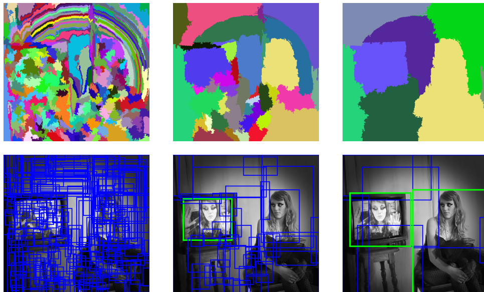
Figure 2.3: Process of extracting region proposals using the Selective Search algorithm. The first image in the top row illustrates the initial segmentation step of the algorithm, while the other two images depict the subsequent merging of regions. The bottom row images illustrate the final step, where each region is assigned a bounding box. Each image depicts the result corresponding to the segmentation state shown in the respective image in the top row. It is important to note that the color specification of the bounding boxes is irrelevant for this explanation. [7]
