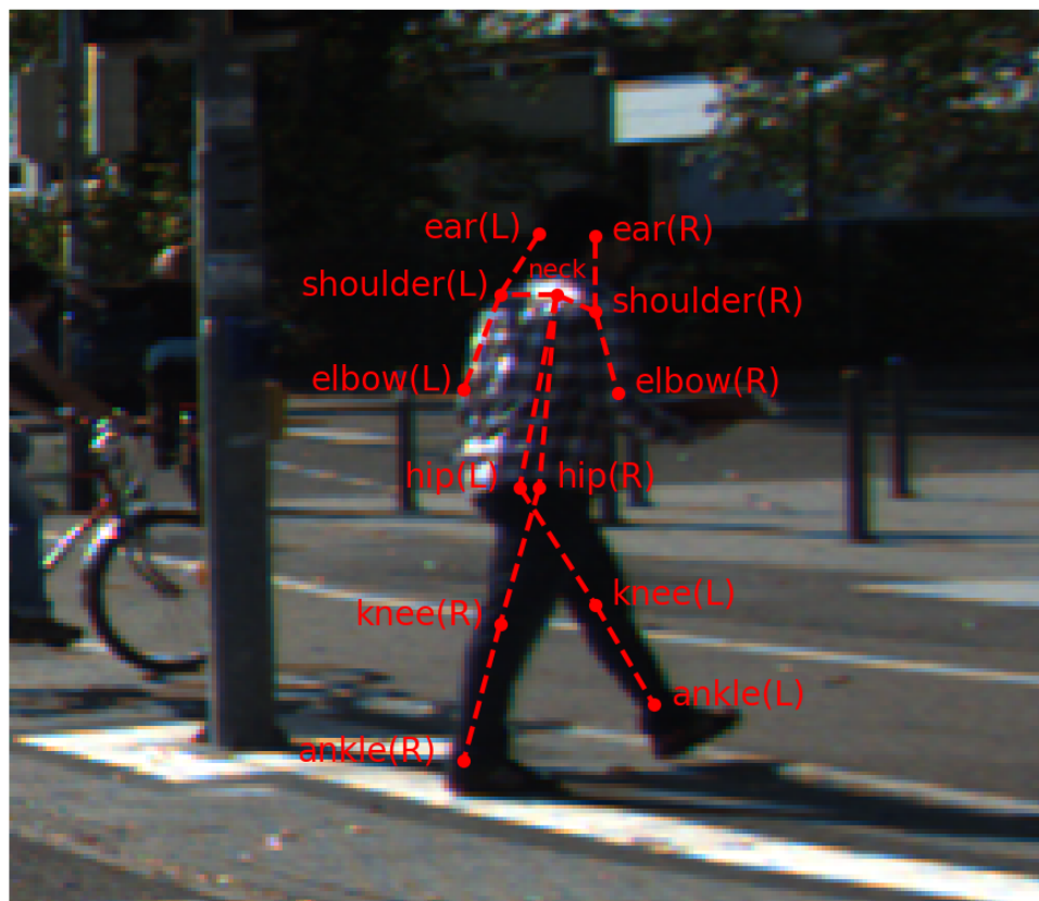
Figure 3.4: Pose estimation for a pedestrian showing 12 estimated keypoints. Dataset specifications: [Sequence: 15, Image: 100, Pedestrian ID: 5]
