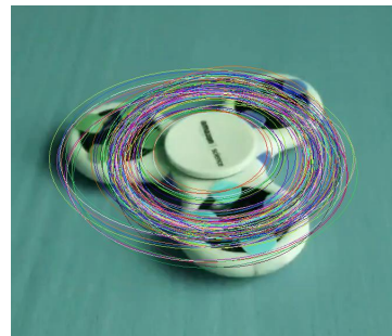
(b) Fitting ellipses for the trajectories of the rotation points for a video shot at approximately 45 degrees to the axis of rotation of the object.
