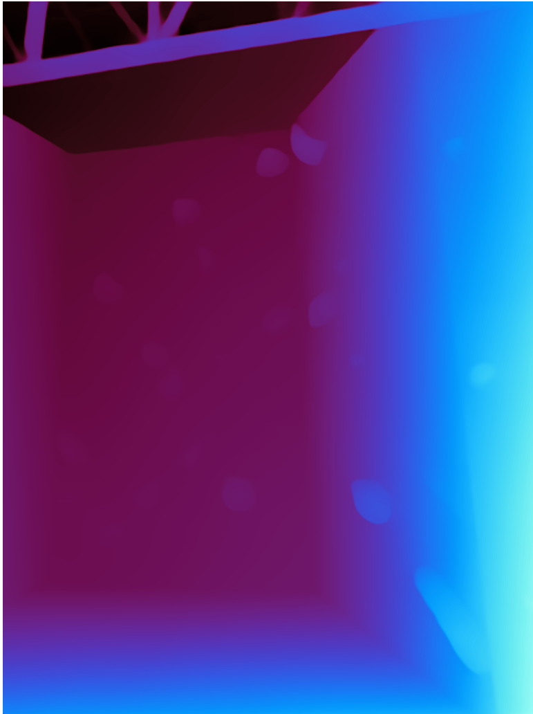
Figure 2.2: Depth-Anything [22] result from a single image (a model based monodepth algorithm approximates depth without any other data.)
