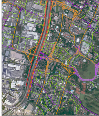
Site visited on January 24 Legend: - Highway system - Main artery - Minor artery - Feeder road - Service Road Scale: 0 to 0.3 km (0 to 0.3 mi)
