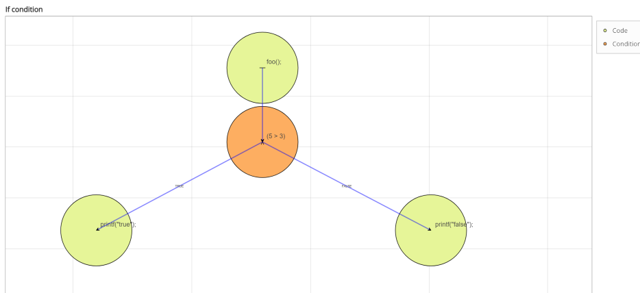
Figure 6.4: Drawing of if-else condition in control flow graph
