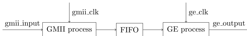
Figure 3.9: Structure of MAC receiver
