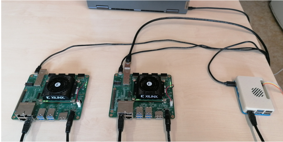
Figure 8.8: Image of sync test setup
