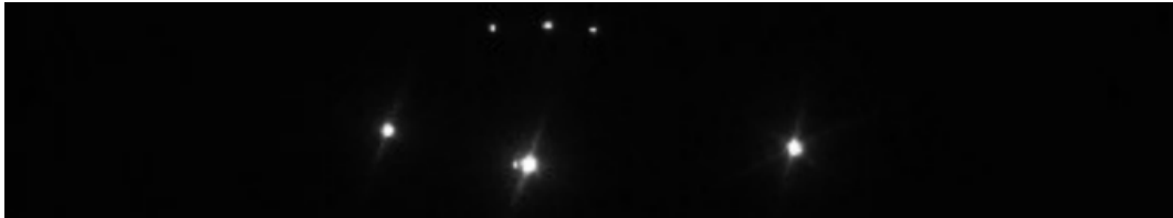
Figure 3.1: The image description, captured by the modified camera, shows two UAVs at varying distances, with "white" blinking UV indicators (Figure 6. in [38]).
