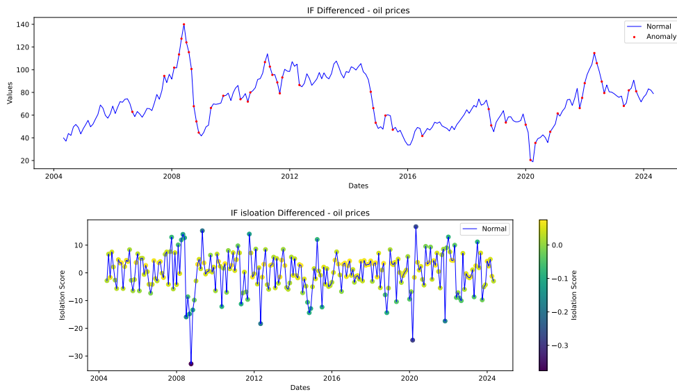
■ Figure 4.5.18 Oil price anomalies and separation score for Isolation Forest with differenced data.
