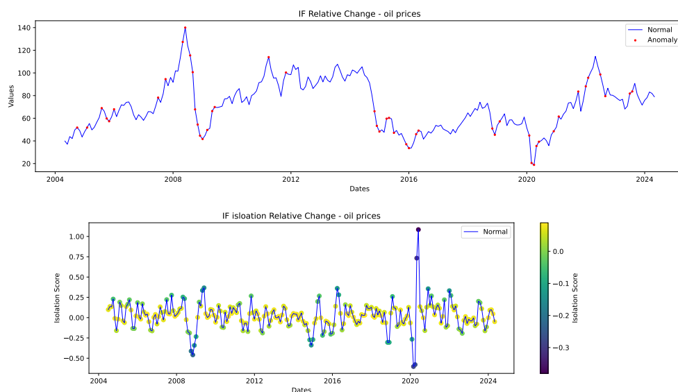
■ Figure 4.5.24 Oil price anomalies and separation score for Isolation Forest with relative change time series.
