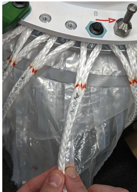
Figure 4.5: Braided Dyneema tendon attached to the apex assembly load ring on Loon super-pressure Balloon [2]
