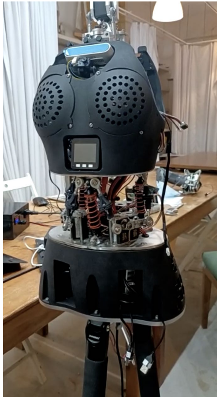
Figure 2.6: Sophia's 6 DoF movable torso prototype. (Source: Hanson Robotics Limited)
