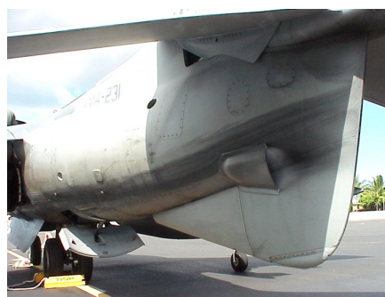
(b) : Detail trysky AV-8B Harrier II na ocasu.
