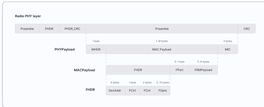
Figure 2.7: LoRaWAN Message Structure [34]
