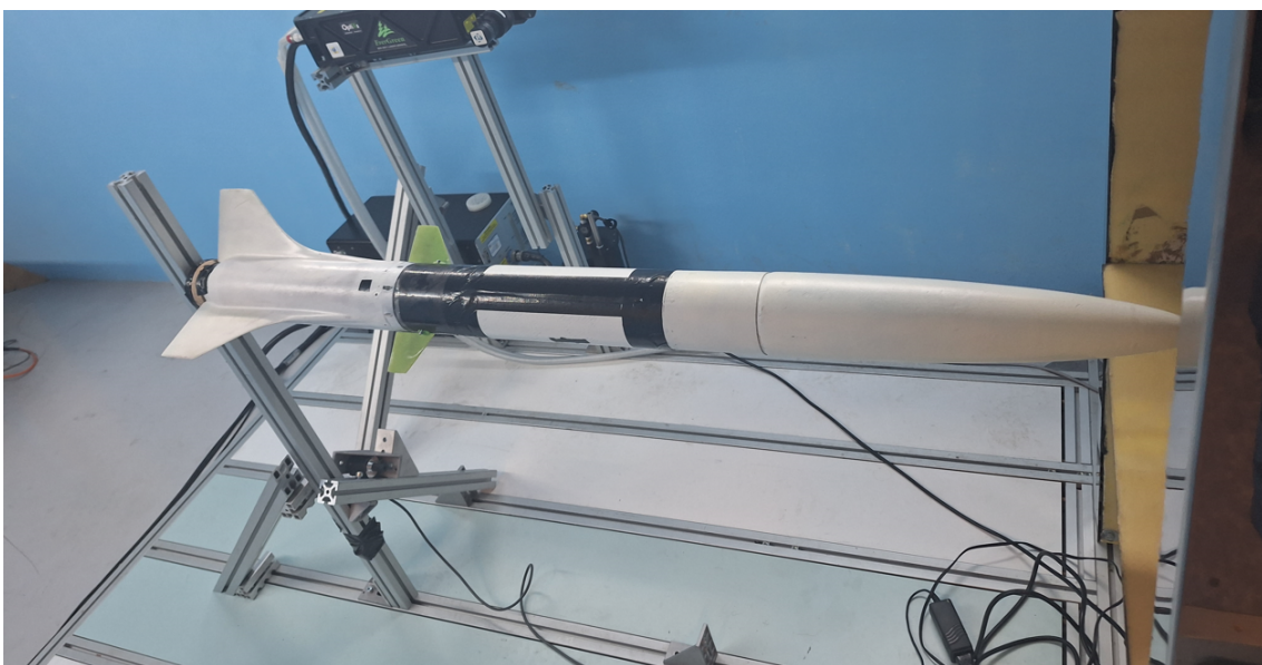
Figure 7.6. Second round of the wind tunnel testing including the larger secondary design of control surfaces.
