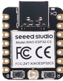
Figure 3.2: Seed Studio XIAO ESP32-C3 board photo [26]
