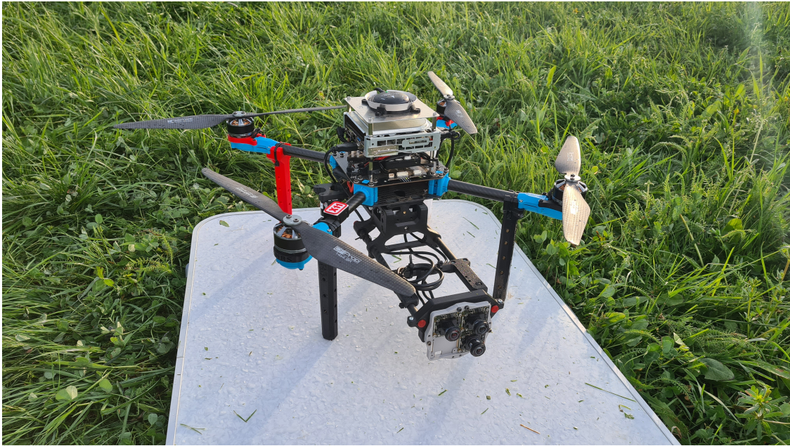
Figure 4.5: The experimented MAV platform at the launch location equipped with three Bluefox cameras.
