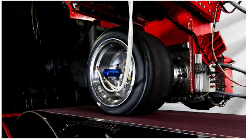
Figure 3.5: Calspan tire testing machine
