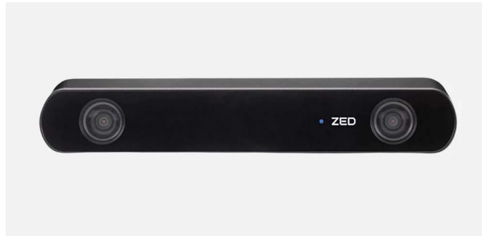
Figure 3.4: StereoLabs Zed2 camera with 2 sensors visible[17].
