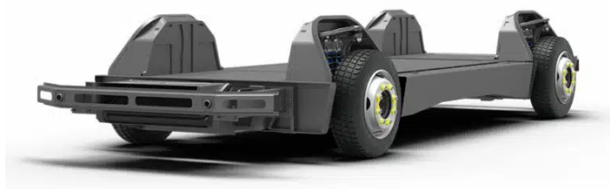
Figure 1.3: Modular REE automotive platform utilizing 4 REEcorner units[3].
