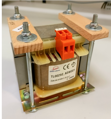
Figure 2.10: Photo of the 1.15H inductor used for inductive load tests in the Siemens laboratory
