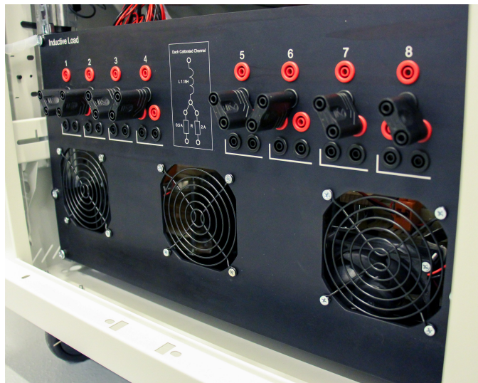
Figure 2.31: Finished panel of inductive load (9) mounted on the front side of station
