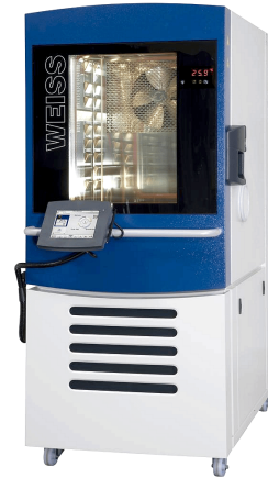
Figure 2.5: Laboratory climatic chamber WEISS-WK3 180/70, source: [1]
