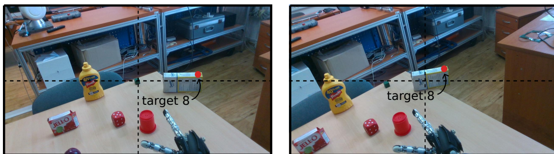
Figure 5.9: Gaze control experiment on the real robot. Position of Target 8 before (left) and after (right) gaze control. The dashed lines indicate the centre of the FoV.
