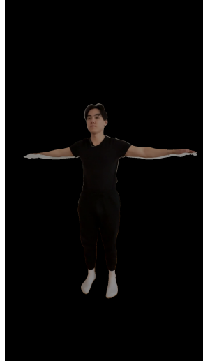
Figure 3.8: The figure shows an image where outline of a mesh is used as a foreground over an image. Notice how the hands do not correspond with the rest of the outline.
