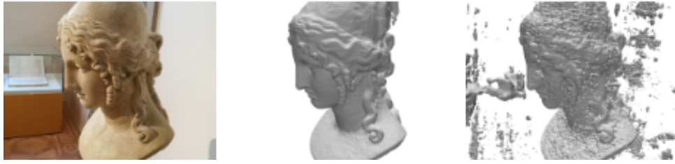
Figure 2.2: Reference image on the left followed by mesh obtained with NeuS and lastly by NeRF. The amount of noise in the NeRF model shows the disadvantage of using purely volumetric rendering for surface reconstruction. Image taken from [49].
