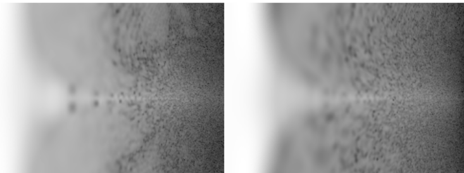
Figure 3.14: Log-polar transform of the magnitude of the frequency-domain images.
