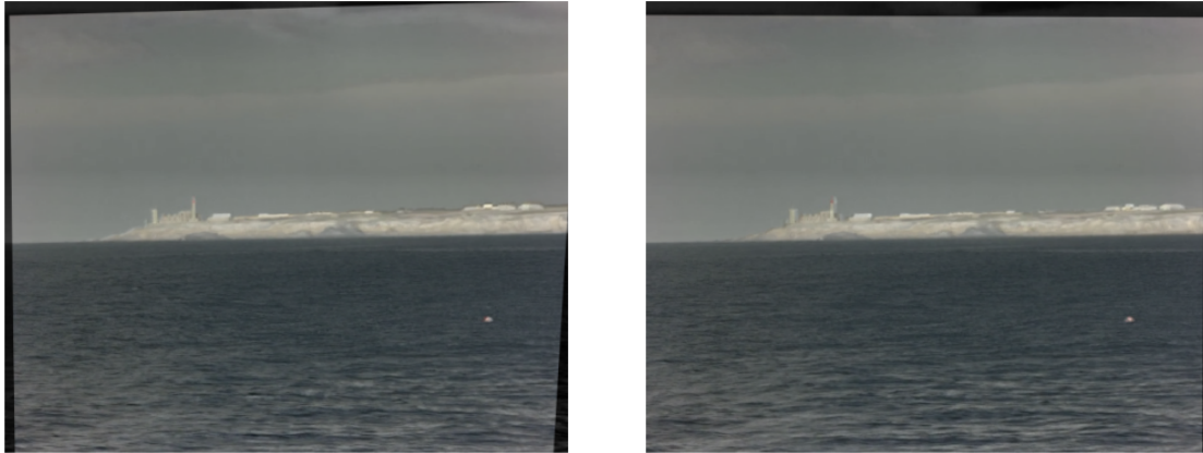
Figure 3.20: Transformations estimated from SP+SG correspondences. General projective transformation is on the left, affine on the right.
