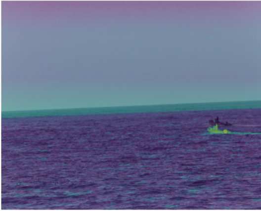
Figure 3.3: Overlapped RGB and thermal images after applying H_{R \rightarrow T} constructed from camera parameters for Sentry.
