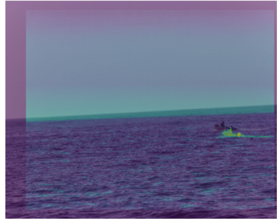
Figure 3.4: Overlapped RGB and thermal images after applying H_{T \rightarrow R} constructed from camera parameters for Sentry.
