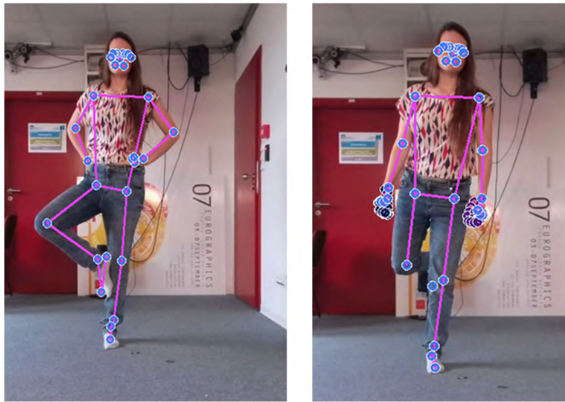
Figure 7.9. An example of typical dataset entry. The image on the left represents an incorrect posture. The image on the right induces correct standing, with hand landmarks (denoted as black circles) detected.
