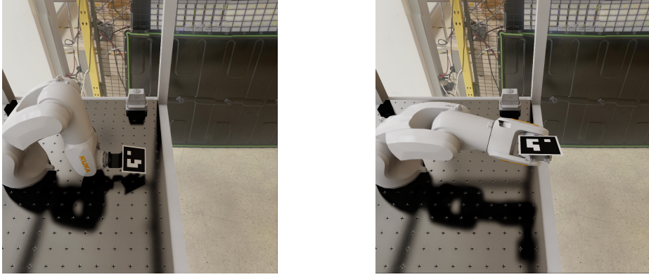
Figure 3.20: Two of eighteen calibration poses from the process of extrinsic camera calibration
