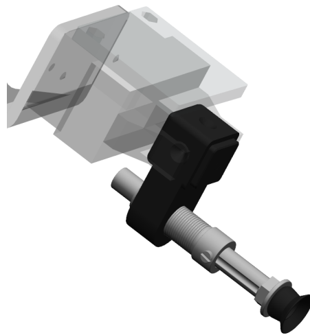
Figure 3.5: Vacuum end effector setup in Process Simulate
